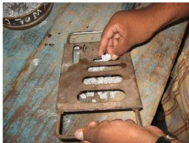
Flakiness Index Test in Progress
