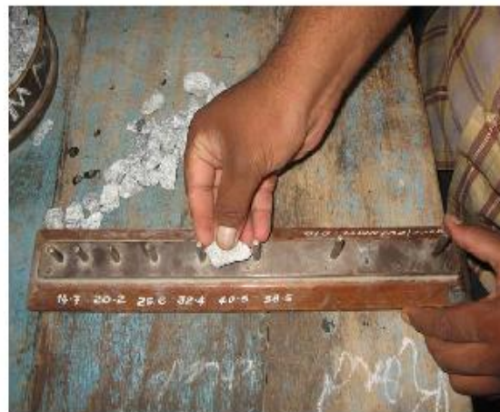
Elongation Index Test in Progress
